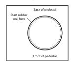
3. Apply a bead of silicone around the top of the rubber seal and at the trimmed join line of the rubber seal.
