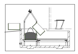
3. The empty basket can now be placed on top of the full basket. The full basket will remain inside the unit for another cycle whilst it's contents dries.
