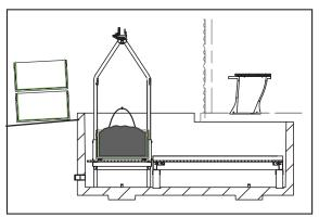
2. Slide the empty basket over the top of the full basket, and slide it directly underneath the toilet bowl. Use the basket Hook tool to maneuverer it into position.
