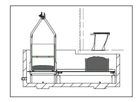
5. Open the Service Door. Remove the empty basket and the basket containing the now partially dehydrated waste from the first service cycle.
