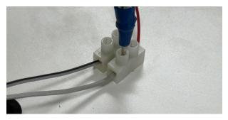
3. Connect the **black striped wire** into the terminal block in line with the **black wire**.
