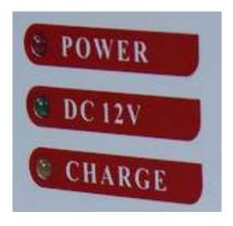
The fan should start to run if the battery is charged. The indicator lights on the front of the UPS should be active depending on the power source (mains power or DC 12V).
