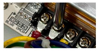
8. Connect the **black striped crimp wire** to the **GND terminal**.
