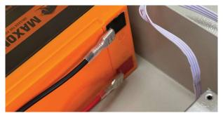
4. Connect **black battery cable** to the **negative terminal** on the battery.
