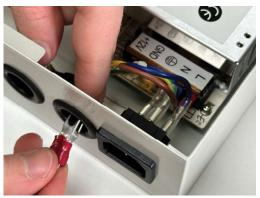
1. Puncture the rubber grommet nearest to the plug on the UPS. Feed the crimped end of the wires through the grommet.
