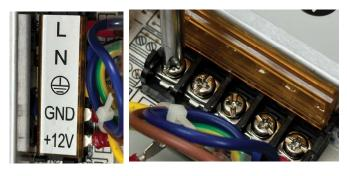
2. Pop open the wire cover. Loosen the two screws for +12V and GND.
