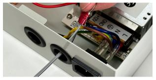
6. Puncture the rubber grommet nearest to the plug on the UPS. Feed the crimped end of the wires through the grommet.
