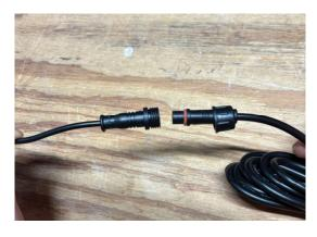
5. Plug in the fan and solar cable via IP rated connector and screw the joining cap to secure.
