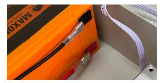
9. Connect **black battery cable** to the **negative terminal** on the battery.
