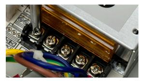
7. Pop open the wire cover. Loosen the two screws for +12V and GND.
