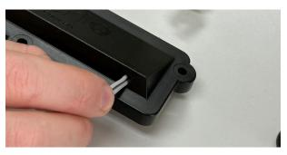
2. Insert the UPS extension wires through the opening near the bottom corner of the fan cover.
