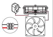
3. Insert the bug Mesh and fan into the housing. Power on the fan to test the connection. Screw the cover onto the fan housing.
