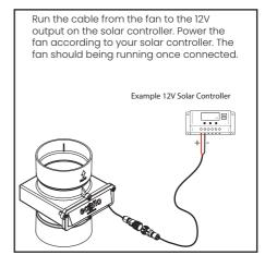
Older models may have the terminal block inside, refer to schematic below. Standard twin core cable can be used.
